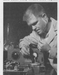
CHEMICAL TEST on an electrical contact is performed by Don Fjelseth. He is placing a very small drop of sodium oxide on the contact surface which will react if sulphide is present.
